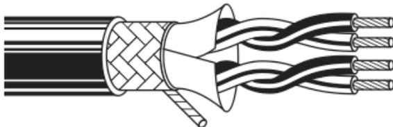
**Braided Shield, Foil Shield, and Twisted Pairs (Image from Belden, [www.belden.com](http://www.belden.com))**
